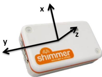
Figure 1: Tri axial accelerometer Shimmer® module is shown above with the directions of three axes.
